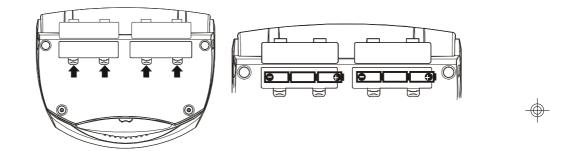
Be sure to observe the correct polarity when installing the batteries. If the batteries are installed incorrectly the unit will not operate.
